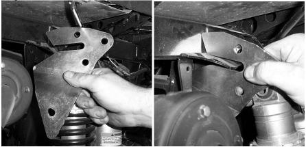
5) You can temporarily hold the bracket in place on the top hole using the 12mm x 75mm bolt.
