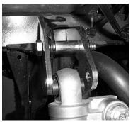
8) Insert the 12mm x 75mm bolt all the way through securing it with the 12mm lock nut.
