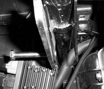
11)Insert the 4Y spacer between the shock mount tabs then push the bolt through the spacer.
