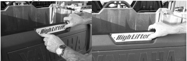
2. Once you find the center, attach the plate to the tail gate using the self tapping screws provided.
