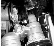
9) Next insert the long front lift bracket into the frame starting from the driver's side of the UTV. Insert the bracket so that it is to the rear of the shock mount and to the outside of the shock mount. Also, insert the bracket with the notched side down and so that it is on the right side of the UTV. The notch is designed to clearance the bracket from the voltage regulator.
