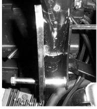
12) Connect the smaller front lift bracket towards the front on the outside of the shock mount tab.
