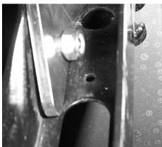
7) Next you will need to insert the 47X spacer between the shock mount tabs and you will also need to insert the smaller rear lift bracket between the shock mount tabs but towards the front.
