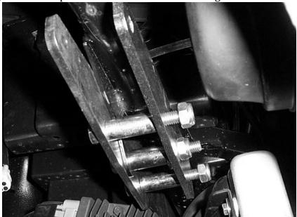
17) Connect the top of the shock to the lift brackets. Place 2ea 10mm washer on both sides of the shock eyelet. Secure the brackets, washers, and shock eye using a 10mm x 70mm bolt and 10mm lock nut.
