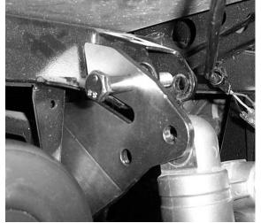
6) The lower portion of the bracket needs to be connected to the frame. Use the 10mm x 25mm bolt and 10mm lock nut to connect the bracket to the frame.
