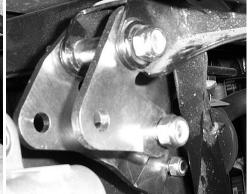
10)Next connect the top of the shock to the lift brackets. Use a 12mm x 70mm bolt and 12mm lock nut to secure the shock to the brackets.
