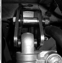
9) Insert the 4X spacer between the two rear lift brackets, securing it with the 12mm x 70mm bolt and 12mm lock nut.
