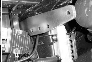
10) Starting from the right side insert the 10mm x 70mm bolt through the bracket and shock mount tab.
