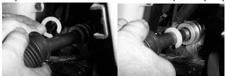
6) Pull boot back over the ball joint and steering stop and refasten with zip tie. Be sure to verify the zip tie is tight so prevent material from getting into the boot.
