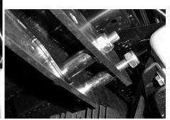
15) Now insert a second 9Y spacer between the two brackets, this time to the outside of the UTV, but not on the ends of the bracket. That position is used for the shock.
