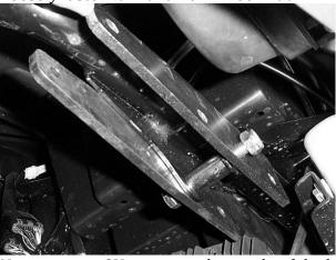
14) Next, insert a 9Y spacer to the inside of the lift brackets closest to the frame. Secure the spacer between the brackets using a 10mm x 70mm bolt and 10mm lock nut.
