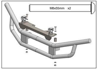
4. Set the two 1" spacers on the bumper holes. Then set the mount on the bumper and attach using (2) M8 x 55mm Hex Bolts, two 1" Spacers (J), six washers, and two M8 Lock Nuts. The order is shown in the picture above.
