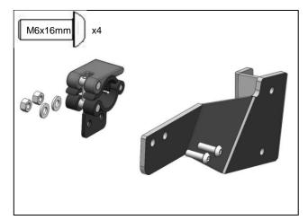
6. Attach the two Rear Clamps (E) To the Hood Rack Bracket (F) with two M6 x 16mm socket head bolts, 4 washers and 2 nuts. The clamp lever should open towards the front of the vehicle.
