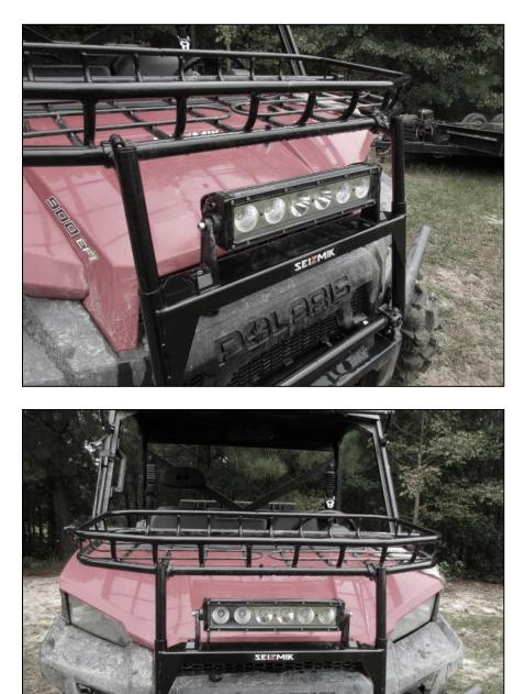
Lights or a light bar can be attached to the hood rack by drilling holes in the light mounting plate. We recommend our 13" 60 Watt Siezmik Light Bar with 5,400 Lumen output. Part Number #12037
