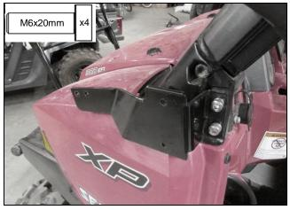
5 Attach the hood rack brackets (F) to the sides of the roll cage using (4) M8 x 20mm socket head bolts as shown above.
