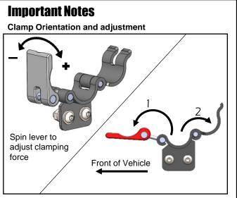
To open a clamp, lift up on both levers in the order above. Orient all clamps so the first clamp lever opens towards the front of the vehicle. To increase clamping force, spin the lever clockwise; to decrease the clamping force, spin the lever counter-clockwise before locking.
