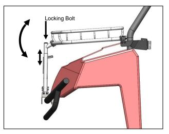
9. Adjust the width of the extendable tubes (G) so they stick out just past the clamps. The hood rack angle can be adjusted by loosening the bolt on the front riser stems and lifting up or pushing down on the front of the rack. Adjust clamps and brackets as necessary, then tighten all bolts. We recommend no more than 5% of slope to the hood rack.
