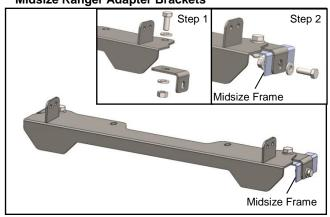
NOTE: Follow these instructions for the MIDSIZE ranger Step 1. Hand tighten (2) M8x20mm bolts, washers and locknuts to secure the Midsize Adapters (J) to the bumper mount. Step 2. Place bumper mount with adapter brackets on the midsize bumper. Line up the holes on the Midsize frame and secure with (2) M8x20mm bolts. Tighten all 4 fasteners. Skip this step if you have a full size ranger.
