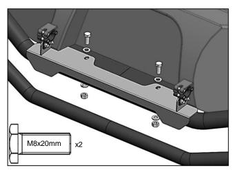
4. Set the mount on the bumper and securely tighten using (2) M8x20mm Hex Bolts, 4 washers, and two M8 Lock Nuts. It may be helpful to remove the plastic grill above the bumper (secured with two torx bolts) for easier access to the nuts. If you have midsize ranger, see note above.
