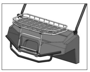
8. Attach the assembly to the front of the hood rack and bolt the two front riser caps in place. Snug the cap bolts, but keep them loose enough to allow rotation. Make sure all 4 clamps are open, then set the rack in place.
