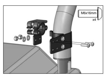
6. Attach the Rear Clamp (E) to the Hood Rack brackets using (2) M6 x 16mm bolts, (2) washers, and (2) locknuts as shown above. The clamps should open towards the front of the vehicle.
