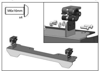
3. Attach the two front clamps to the bumper mount using (4) M6 x 16mm bolts, (2) washers and (4) locknuts. Make sure all clamp levers open away from the vehicle.
