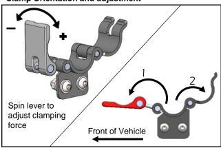
To open a clamp, lift up on both levers in the order above. Orient all clamps so the first clamp lever opens towards the front of the vehicle. To increase clamping force, spin the lever clockwise; to decrease the clamping force, spin the lever counter-clockwise before locking.
