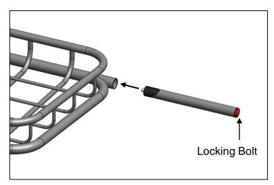
2. Insert an Extendable Tube (G) in each end of the hood rack. Push in just a few inches and tighten the locking bolt in the end of the tube just enough to hold the extending tube in place. You will make a final adjustment and tighten later.
