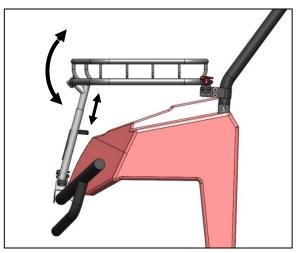
9. Adjust the width of the extendable tubes (G) so they stick out just past the clamps. The hood rack angle can be adjusted by loosening the bolt on the front riser stems and lifting up or pushing down on the front of the rack. Adjust clamps and brackets as necessary, then tighten all bolts.
