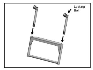
7. The picture above shows the riser orientation for the full size and midsize. Note your vehicle's orientation. Insert the 2 Front riser stems into the front riser/light mounting plate a few inches in. Tighten the locking bolt at the top of the tube just enough to hold the riser stems in place. You will tighten after final assembly.
