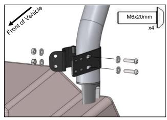
5. Install the Hood Rack Brackets (F) to the front roll cage with two M6 x 20mm socket head bolts, (4) washers and (2) locknuts for each side. Point the bracket towards the front of the vehicle. Do not fully tighten bolts yet as you may need to adjust when you put the basket in place.
