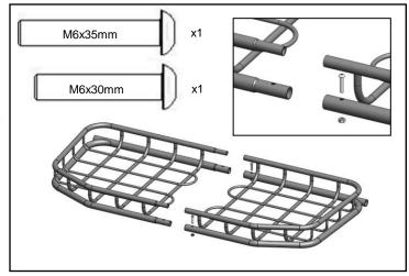
1. Assemble two sides of rack (A). Secure the larger rear tube with an M6 x 35mm Socket Head bolt and lock nut. Secure the front smaller tube with an M6 x 30mm Socket Head bolt and lock nut.
