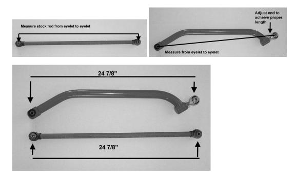
11. Once you have set the distance on the new rod attach it to the RZR. Attach the ends of the radius bars to the RZR frame using the 10x65mm Hex Bolts, 10mm Flat Washer provided and the stock flat washer, and 10mm Lock Nuts provided in the kit.
