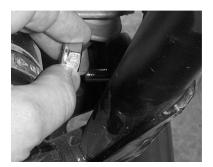
12. Connect the new Heim Joint and Heim Adapters to the knuckle assembly using the stock hardware.
