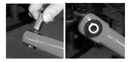
4. Now thread the jam nut onto the heim joint. Run it all the way down to the bottom of the threads and screw the heim joint into the radius bar
