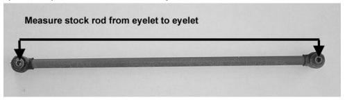
9. Set the distance on the new rod by adjusting the heim joint and jam nut.
