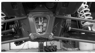
8. When you have removed the rods you will need to take a measurement of the rod. Measure from eyelet to eyelet. You will need to adjust the new radius rod to this distance.
