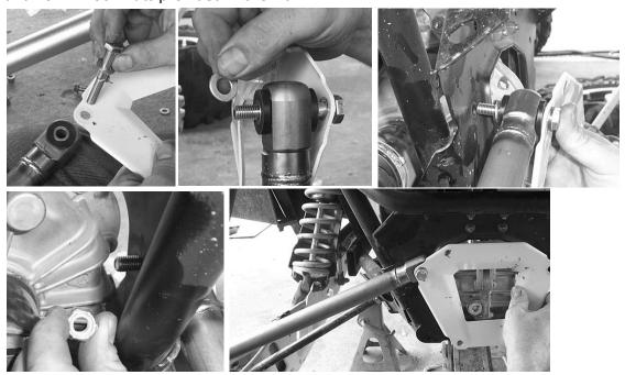
11. Connect the new Heim Joint and Heim Adapters to the knuckle assembly using the stock hardware.
