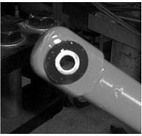
4. Now thread the jam nut onto the heim joint. Run it all the way down to the bottom of the threads and screw the heim joint into the radius bar
