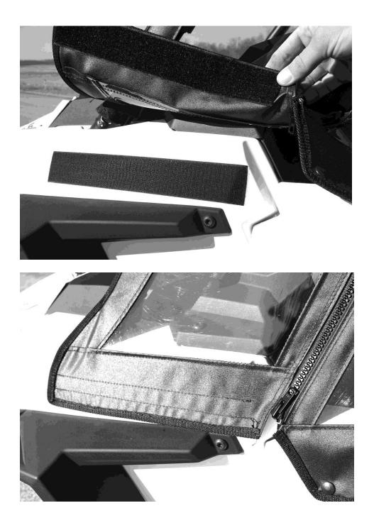
d. Lastly snap the bottom of the door to the plastic doors on the RZR. NOTE: it helps to place the screw snaps into the sockets on the cabs first, then starting at the top one, push them into the plastic so a small dimple is left behind. Then pull the screw snap back out and screw it into the plastic where the mark was made. See photo below
