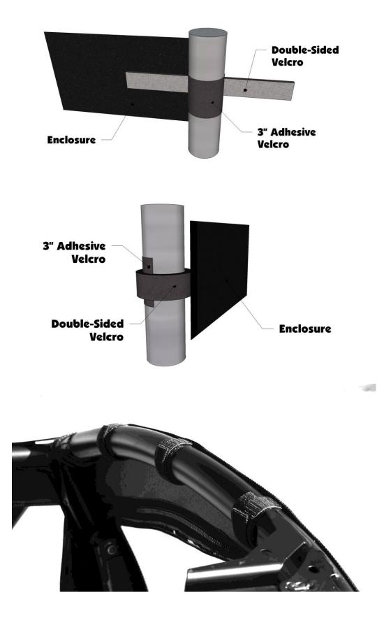
b. After installing the double-sided strips move to the rear of the door and attach the two Velcro tabs to the rear bar using the corresponding adhesive Velcro strip. See Photo Below:
