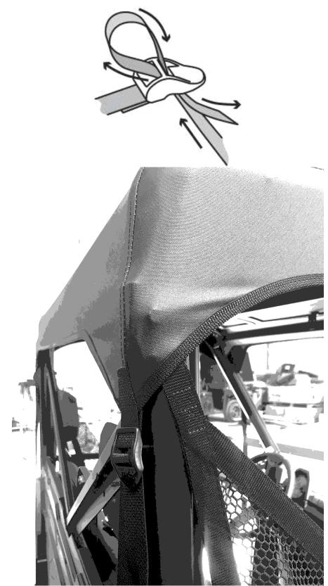
• Moving to the front of the vehicle you will now need to raise the hood to reveal frame. Again take the looped end of one of the straps and run it around the frame
