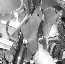
11. Connect the top of the shock to the lift plates. Insert the 10 x 70mm hex bolt through from the backside forward. Place a small **Spacer JJ** between the shock eyelet and the lift plate. Fasten it tight using a 10mm lock nut provided.
