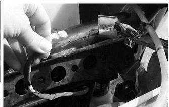
4. Run the wires behind the cross member on the frame and reconnect to the lights.
