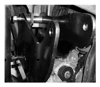
8. Connect the second 10mm x 55mm bolt into the lower portion of the lift bracket and loosely connect the bolts using the 10mm lock nut.
