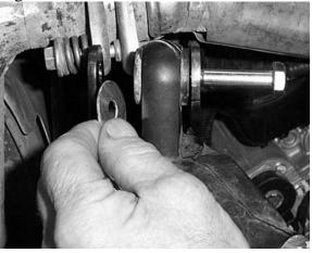
10. Once you have placed the fender washer on the bolt, place the **NNN Spacer** onto the bolt, and then fasten the bracket to the shock using the 10mm lock nut.
