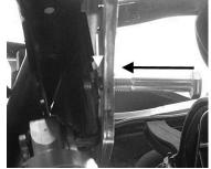
8. Next insert **Spacer O** in the stock shock mount position and push the 10x70mm bolt through. Repeat steps for the opposite side at this time.
