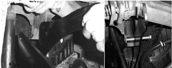
7. Place the **F Spacer** on the outside of the shock mount tab and now place the right outer bracket in place. Loosely connect it using the 10mm lock nut.
