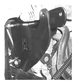
9. Connect the top of the shock to the brackets using the 10x80mm bolt and 5/16" fender washer.
