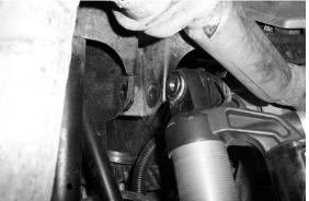
4. Starting from the passenger's side, rear right from the seated position; insert the inner right bracket into place **between the shock mount tabs**. But first place a 10x55mm bolt through the lower portion of the bracket. It is going to be very difficult to insert this bolt if you do not install it first. Now insert the bracket
