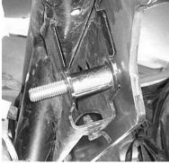
9. Insert the front slotted bracket on the backside of the front cross member.
