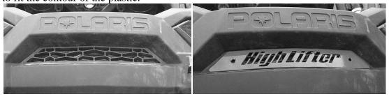
3. Using the two button head bolts, washers, and lock nuts to connect the plate to the plastic.
