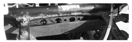
7. Insert the 10 x 70mm bolt through the bracket, placing a 10mm washer between the bracket and the shock mount.
