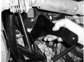
5. Connect the outer rear right bracket to the bolt and secure it loosely with the 10mm nut.
