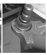
6. Use the factory nuts and bolts to connect the new Control Arms to the RUV frame. You will have left and right lower Control Arms.
