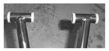
NOTE: A press or a vise is suggested for removing and replacing the ball joints. Verify that the clip snaps into place after installing the ball joints into the new Control Arm
