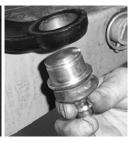
5. Install the grease fitting into the new arms before installation. Install the fittings in the new arms like they are in the factory arms. DO NOT OVER TORQUE THE FITTINGS. Make sure to fill with factory approved grease.
