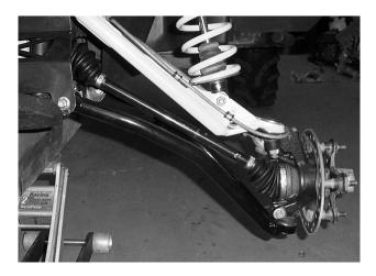
10. Once you have placed the wheels back on the ATV, have someone turn the steering wheel to full lock, left and right, to verify clearance between all components. There should be no interference between the tie rods, hubs, or control arms.
