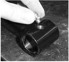
6. Now reinstall the bushings, sleeves, and ball joints into the new arms. If you place some grease on them it makes the installations easier.
