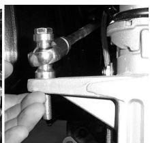
15. Place a second 10mm washer onto the bolt and secure it with the 10mm nut and then the 10mm lock nut.
