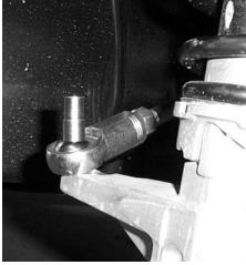
13. Place alignment cones onto the sleeve, on either side of the heim joint.
