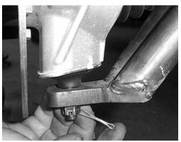
10. Remove the stock tie rod end and connect the new heim joint provided.
