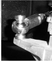
14. Place a 10mm washer onto the knuckle assembly and insert the 10mm x 80mm bolt through the heim joint, sleeve, and cones.
