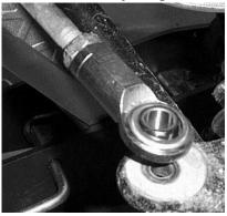
11. To connect the new heim joint to the knuckle assembly use the 10mm x 80m bolt, heim sleeve, alignment cones, 10mm washers, 10mm nut and 10mm lock nut.
