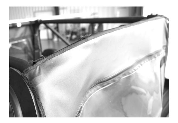
5. Now take the bottom of the door and pull it down so all the magnets are in the proper place.
