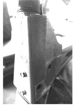
3. Take the door and attach it to the roll cage so the double-sided tab along the back of the door and the 6" tab on the front of the door line up with the adhesive strips you just installed.
