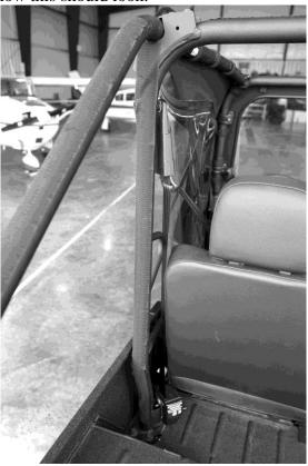
2. Next place the 6" adhesive Velcro strips on the front of the roll cage where the windshield bolts on. Place the strip just above the bottom hole making sure you don't cover the holes up. See photo below.
