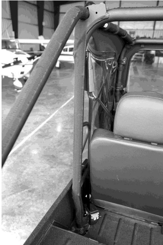
2. Now take the remaining 45" adhesive Velcro strip and run it across the top of the top rear bar as shown in the photo below.
