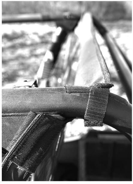
3. Now work your way down each side of the Rear Window attaching the double-sided Velcro strips to the center side bar as shown in the photo below. **NOTE: The Rear window is designed to leave most of the center side bar exposed so the magnets in the doors hold as well as possible so don't pull the sides of the Rear Window too hard.**
