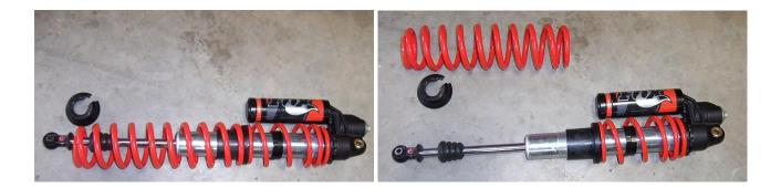
6) Place the front spring spacer to the shock.
