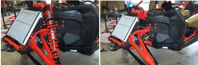
5) Disassemble the shock. If you have not loosened the spanner nut do it now.
