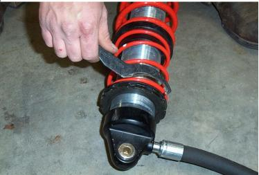
5) Now placing a little pressure on the springs, pull the springs back to release the retaining clip/dust shield. This will allow you to remove the springs.
