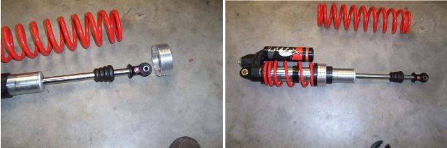
Reassemble the shock by placing the factory spring and retaining clip back onto the shock. You will need to compress the factory spring to reassemble. With the added height of the spring spacers, it requires compressing the springs to reassemble the shock.
