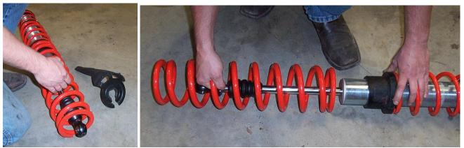
7) Now place the rear spring spacer on the shock.
