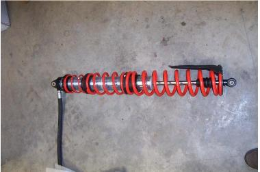
4) Next release the tension on the shock by adjusting the spanner nuts all the way to the end of the threads on the shock. **NOTE: Mark the setting on the spanner nut so you can adjust back to this position when you have installed the lift.**
