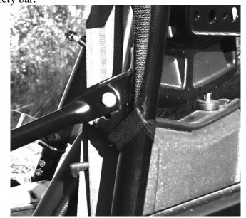
5. Now place the top over the entire vehicle, the front of the top is identified by the sides not being as steeply curved, and begin by lacing the front straps through the ladder lock buckles sewn to the front corners of the top. Diagram below shows how to use ladder buckle.
