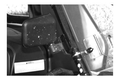
4. Next take the other two straps with a loop sewn on one end and wrap them around the roll cage in the rear just under the safety bar.
