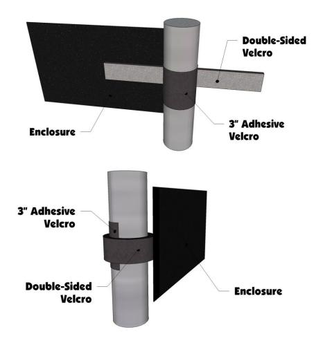
3. The sides of the Rear Panel will attach using the 6" and 12" adhesive strips. (NOTE: The top Velcro strip on the sides may be a tight fit between the bars but will work just fine.) See photo below
