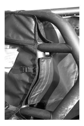
4. Make sure that the Rear Window is centered correctly and then move to the bottom of the panel and take the straps down and around the side bars and then up and through the ladder lock. Do NOT pull them too tight because when the seats are replaced they will be pushing on the rear window. See photo below:
