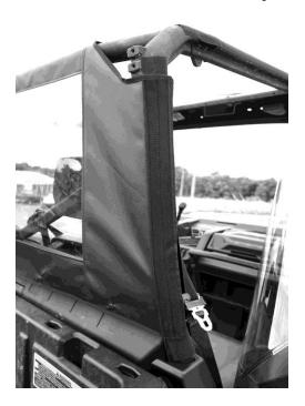
7. Then install the snap studs in the plastic along the bottom of the Rear Window. NOTE: It helps to put the snap studs into the sockets in the canvas first. Then one at a time push the screw into the plastic hard enough so that a mark is left behind. Pull the snap stud back out of the door and screw it into the plastic where the mark was made. snap the door in place and move on to the next one. See photo below
