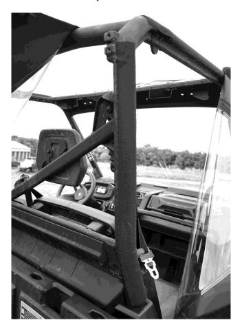
5. Then place the 40" adhesive Velcro strip on top of the of the rear horizontal bar making sure it is centered properly. After that attach the top of the Rear Window here. See photo below
