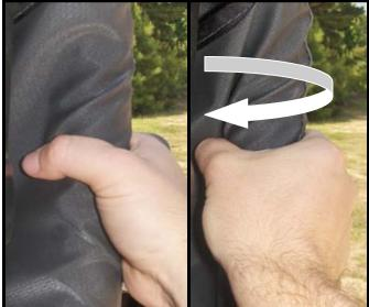
2. Locate the velcro straps running down the length of the rear vertical ROPS bar. Fasten around the bar. Repeat this step for the opposite side.
