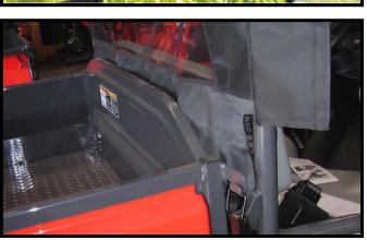
4. Allow the back side to drape between the dump bed and the seat.
