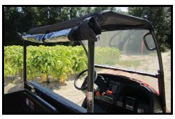
A - The rear window can be rolled up by undoing step 2, rolling the window up from the bottom, and securing with the three straps at the top of the window as shown.
