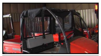
1. Lay the soft top over the roll cage of the vehicle making sure the straps are on the outside of the ROPS.
