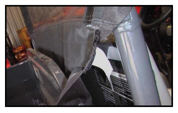
5. Locate the velcro at the base of the soft top with the adhesive velcro strip. Remove the backing to the adhesive and adhere to the horizontal rectangular bar behind the seat..
