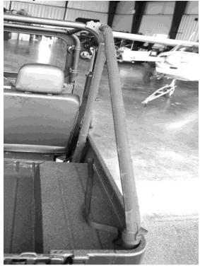
2. Now just line up the top corner so it overlaps the Velcro sewn to the outside of the door and attach it to the door and the roll cage. Pull it down so the magnets are on the sides of the bed and that it. See
