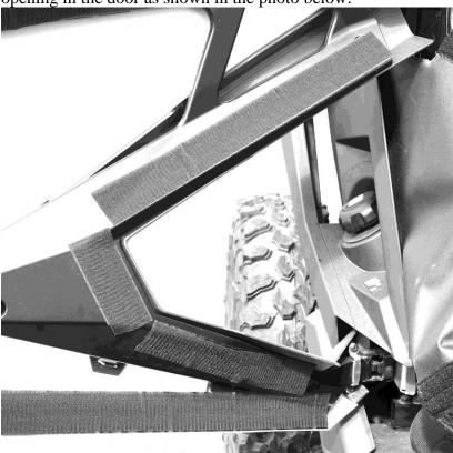
2. Then attach the door insert to the inside of the door as shown in the following photo.
