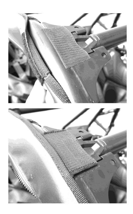
c. Now move to the bottom of the door. In the rear you will see a strap and buckle that will go down and wrap around a bar and back up to the buckle.
