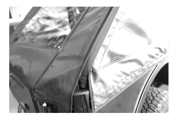
11. Once all the straps are in place run them through the buckles. Pull them tight making sure the top is centered and the side seams line up correctly along the roll cage. The diagram below shows how to lace the webbing through the buckle.
