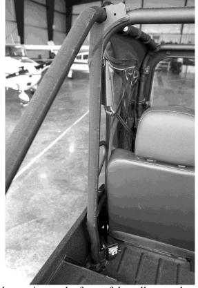
2. Next place the 6" adhesive Velcro strips on the front of the roll cage where the windshield bolts on. Place the strip just above the bottom hole making sure you don't cover the holes up. See photo below.
