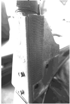
3. Take the door and attach it to the roll cage so the double-sided tab along the back of the door and the 6" tab on the front of the door line up with the adhesive strips you just installed.
