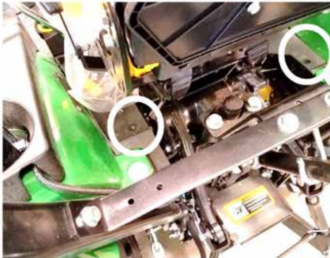
35. Remove the 2 bolts behind the rear seat in the circled area. Do not discard. These bolts will be used in step 41.
