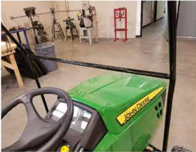
17. Install the windshield cross bar (#8) between the 2 A pillar tubes (#7) using m6x25 button head bolts. Button head must be facing outward.
