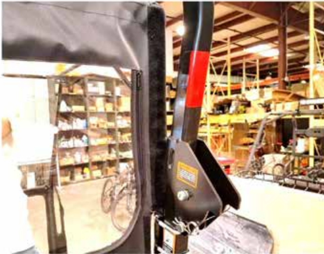
39. Continue from the top, wrapping the side flaps of the rear panel around the rectangular Rops Uprights (#3).
