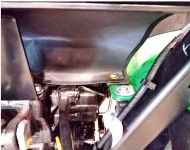
41. There are 2 grommets at the bottom of the rear panel that should line up with the bolt holes from Step 34. Orient the grommets as shown.
