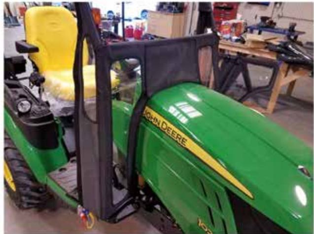
32. Attach the front textile to the frame structure and the quarter panels using Velcro as shown.
