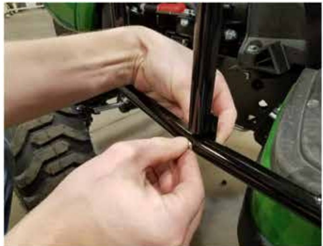
20. Attach the Door Close Tube (#9) to the driver foot pan bracket (#1) with the longer m6x30 button head bolt as shown. Button head must be facing outward.
