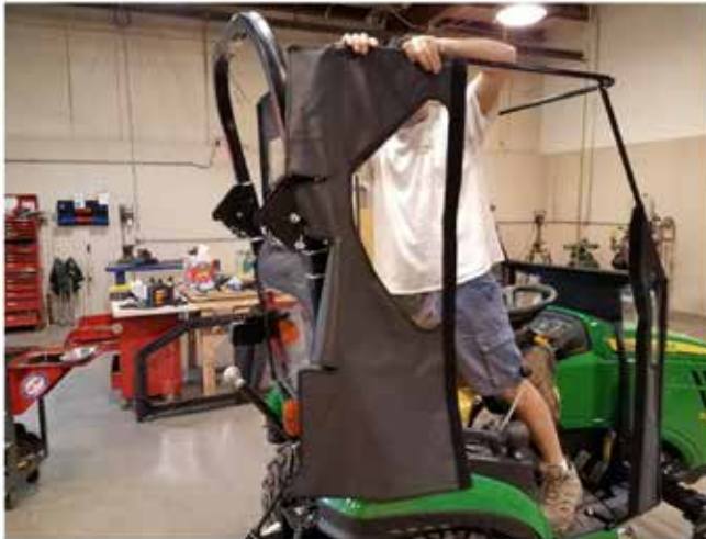
43. As done with the rear panel, start by hanging the right rear quarter panel from the top roof hoop (#6). Secure to roof hoop with flaps so that it hangs as straight as possible.
