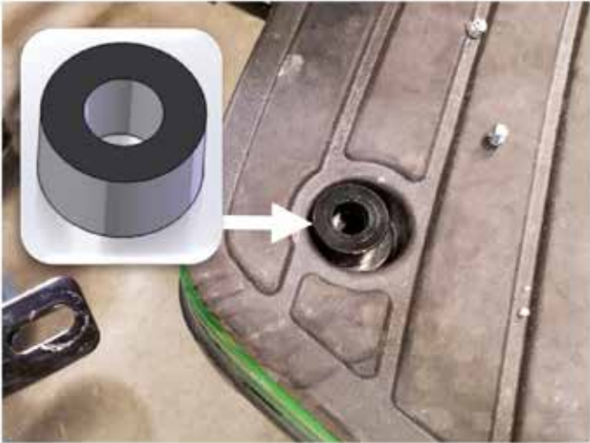
1. Remove the forward most foot pan bolt and place one of the shorter spacers included in the cavity.
