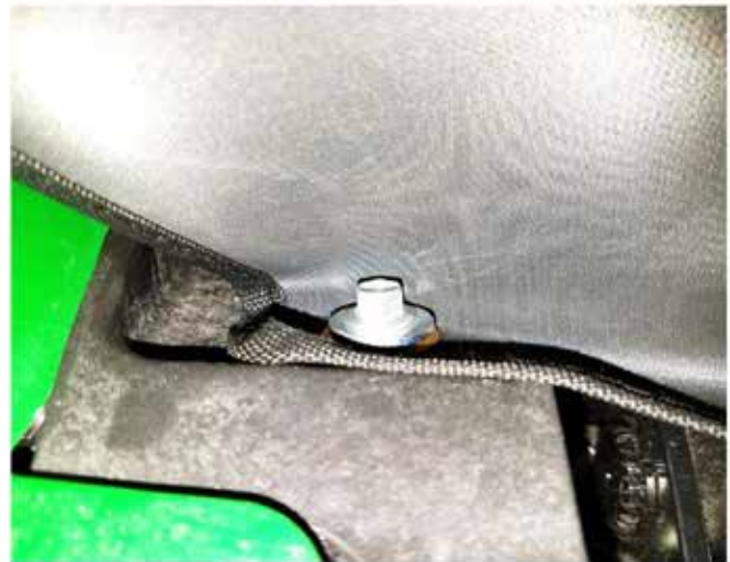
42. Reinstall the bolts removed in step 34 through the grommets at the bottom of the rear panel as shown above.
