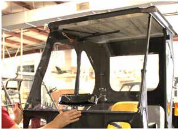
63. Hold the windshield up in position with the upper bend facing forward towards the front lip of the roof.
