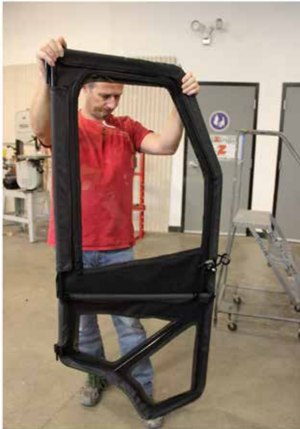
58. Install upper and lower door textiles as shown. It is easiest to install the bottom portion first so that the top can be pulled down tightly and connected to the Velcro on the arm bar flap.
