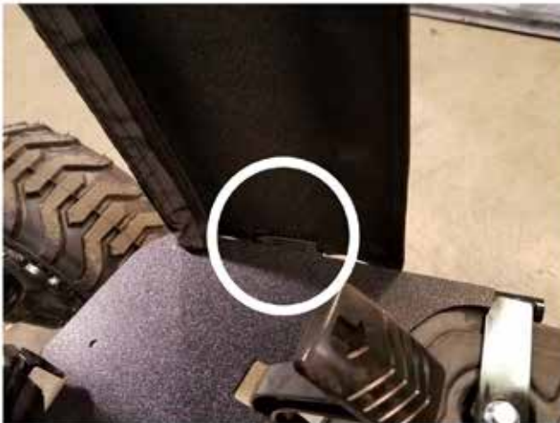
31. Attach the lower flap of the right side quarter panel textile to the foot pan bracket (Green #12) as shown. Tighten down foot plate bolts at this time.
