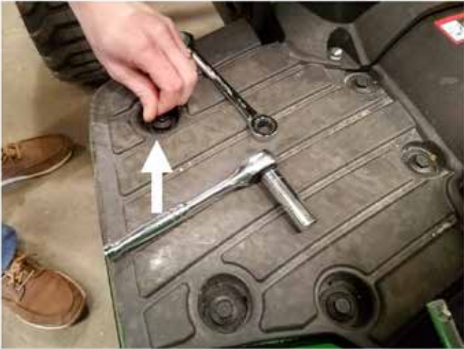
1. Remove the forward most foot pan bolt and place one of the shorter spacers included in the cavity.
