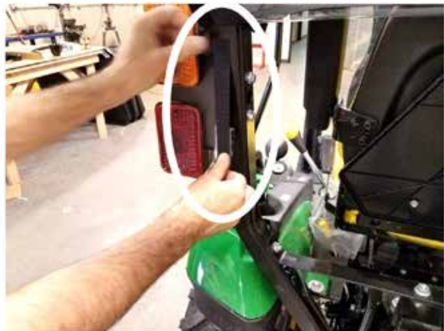
34. Clean the roll over bar in the area shown with alcohol and place a 12" strip of the supplied adhesive Velcro from the middle of the orange tail light downward on both sides. This will aid in securing the rear panel to the tractor.
