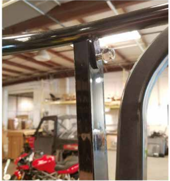
12. Roof hoop (#6) tabs should be on the inside of the rops uprights (#3) as shown above.
