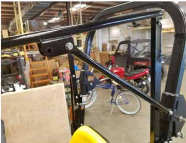
13. On the "drivers" (left) side, attach stay rod (#4) to roof hoop bracket in the rear hole using m8x40 flange bolt as shown. Button head must be facing outward to avoid contact with door.
