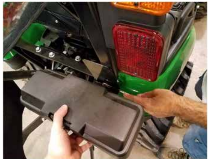
38. Removing the toolbox will make the next few steps of the installation easier.
