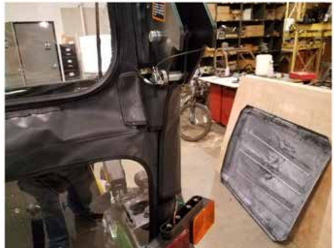
46. The flaps of the quarter panel should line up with the Velcro on the rear panel as shown above.
