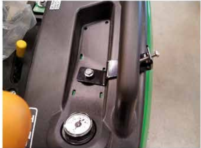
22. Install the fender bracket (#10) in the orientation shown with the supplied M8x40 flange bolt. No spacer is needed for this bracket.
