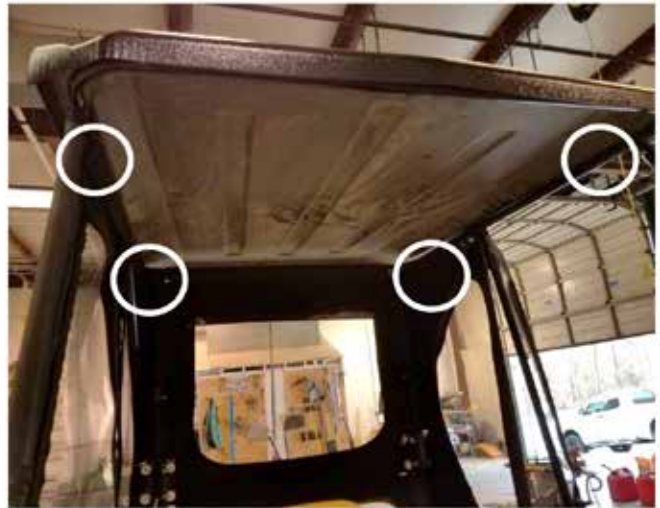
55. The 4 holes are located in each corner of the hoop, circled in the picture above. Secure with Plastic knobs and wing nuts. Holes may need to be poked in the textiles to allow the bolts to pass fully through.
