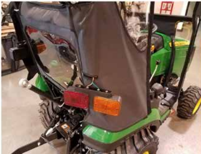
45. With the quarter panel now secured at the top and bottom, secure the remaining flaps around the roll bar structure to the rear panel as shown. The wires for the tail lights should line up with the space between the flaps.
