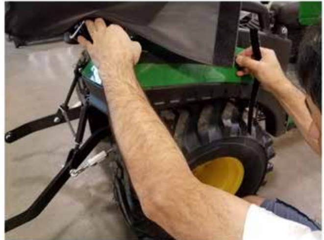
44. With the quarter panel hanging straight, clean the fender with alcohol. Line up the supplied adhesive Velcro with the Velcro at the bottom of the quarter panel and adhere the adhesive Velcro to the tractor fender.
