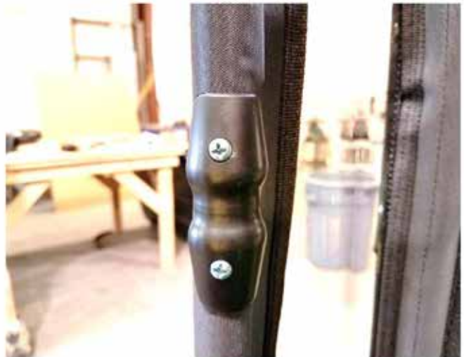
57. With both holes made, screw in the latch lock using supplied sheet metal screws in the orientation shown.
