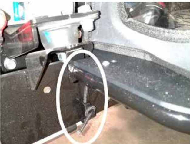
33. The bottom of the front textile is additionally secured to the frame of the tractor using the hooks on the elastic cord on both sides. See picture above. The elastic goes between the frame and the Foot pan bracket (#12) on either side.
