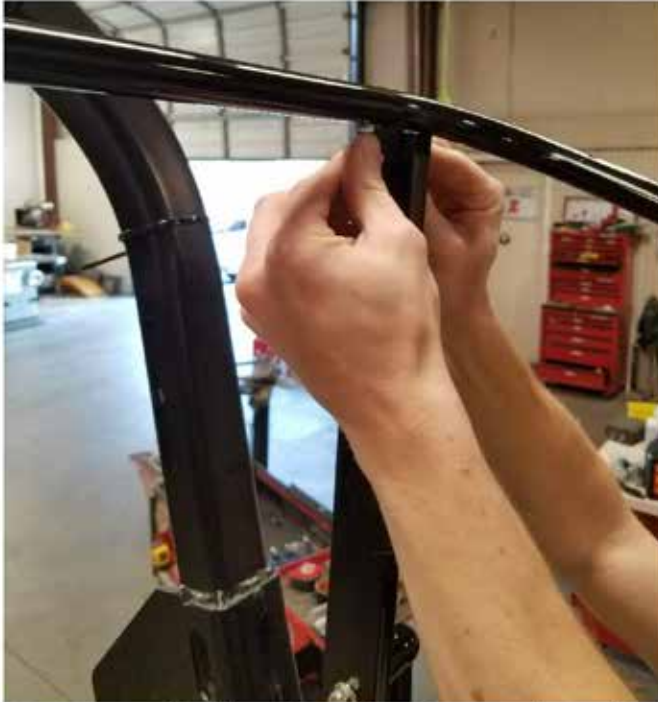
11. Hang Roof (#6) hoop by attaching the rear tabs on the inside of the rops uprights using m8x35 flange bolts. Orient bolts with flange nuts on the inside of the bracket.
