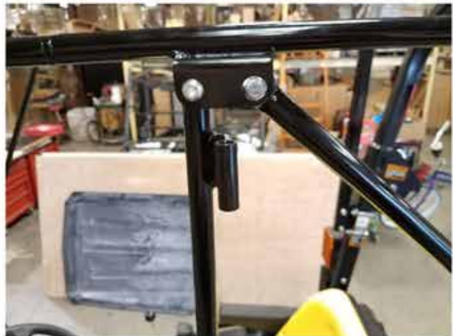
24. Locate the upper portion of the door hinge tube (#11) with the roof bracket in front of the stay rod (#4) as shown in the picture above. Attach with m8x35 button head bolt. Button head must be facing outward to avoid contact with door.
