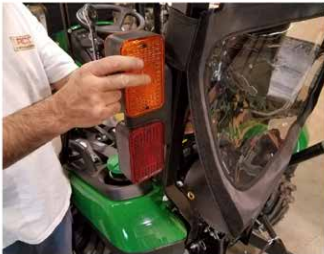
37. If equipped, the rear tail light assemblies will need to be removed for this part of the installation. They will be reinstalled later.
