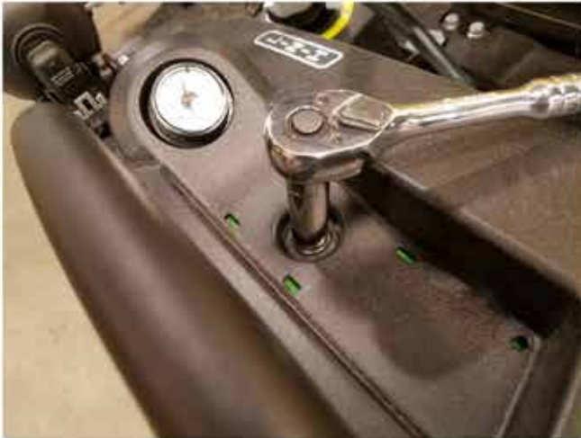
21. Remove the bolt in the "driver" (left) side fender cover in the area shown.
