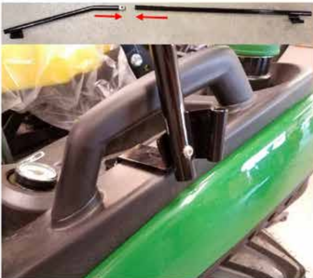
23. Assemble the 2 door hinge tubes (#11a & #11b) with an m6x25 button head bolt and locate the lower hinge tube with the hole in the fender bracket (#10) as shown. Attach with m6x30 button head bolt. Button heads must be facing outward to avoid contact with door.
