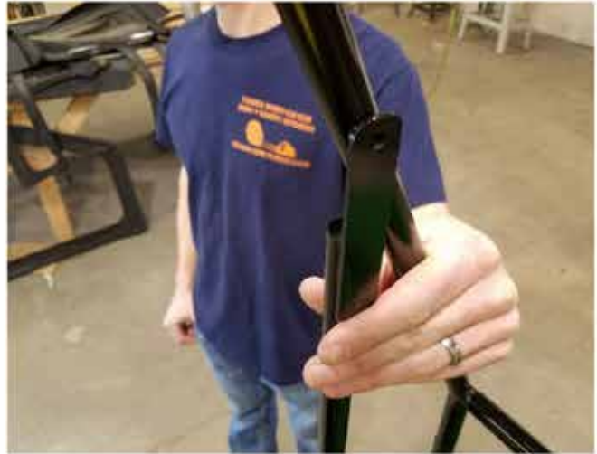
18. Line up the long tab of the Door Close tube (#9) with the hole in the "driver" (Left) side A Pillar Tube (Orange #7). Tabs of the Door Close Tube (#9) should be on the inside as shown.
