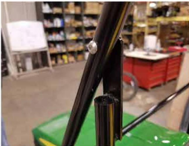
19. Attach upper tab of the Door Close Tube (#9) to the A Pillar Tube (#7) with the longer m6x30 button head bolt as shown. Button head must be facing outward.
