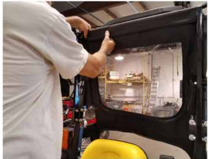
36. Hang the rear panel in the orientation shown by first wrapping the upper flap around the rear of the roof hoop (#6) between the rops and the steel frame structure.
