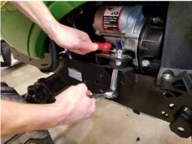
2. Remove the nut from the bottom of the engine mount bolt and place the bent tab of the driver foot pan bracket on the bolt as shown in the pictures above.
