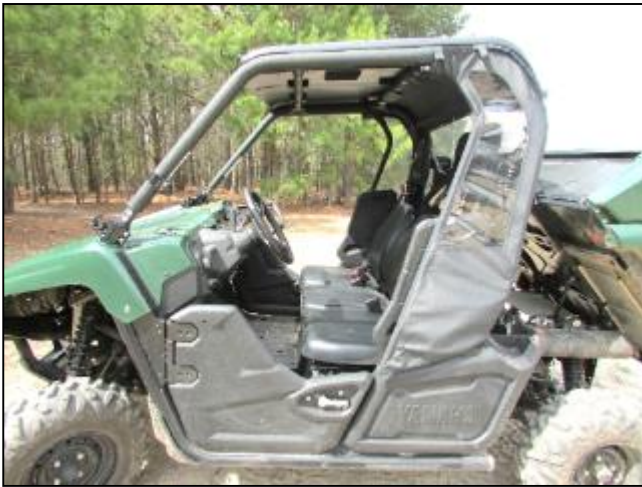
15. Secure the back panel around the Z tube. If needed, refasten the Velcro straps to adjust the fitment of the textiles.
