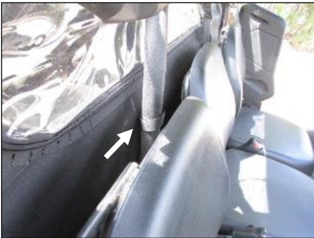
17. Secure the back panel with two Velcro loops around the rear pillars of the cab. There is one behind the passenger and drivers seats.
