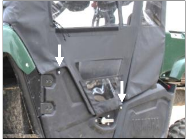
20. Locate the holes on the door based on the door location. Mark and drill through OEM Viking door. Secure with bolts and locknuts.
