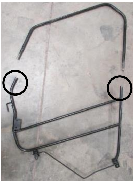
1. Assemble the two halves of the door and secure using two M6x25mm button head bolts.
